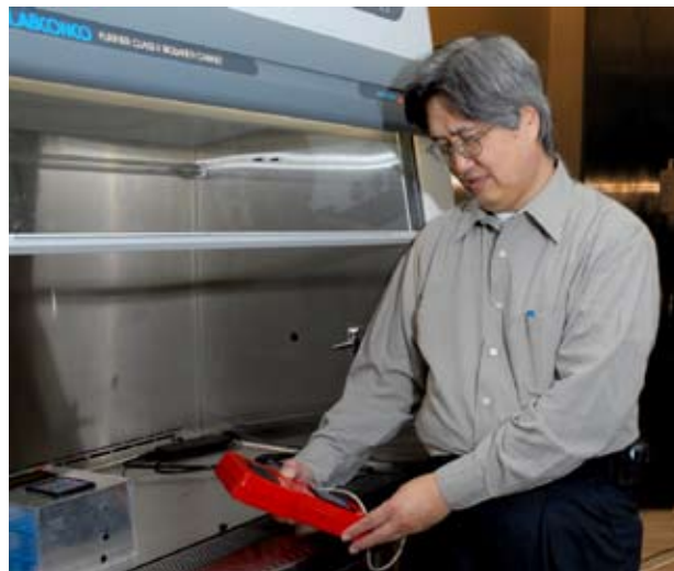
BIOSENSING CHAIR – Yanbin Li with a prototype of a portable biosensor system for field use to rapidly detect the H5N1 bird flu virus in poultry.
