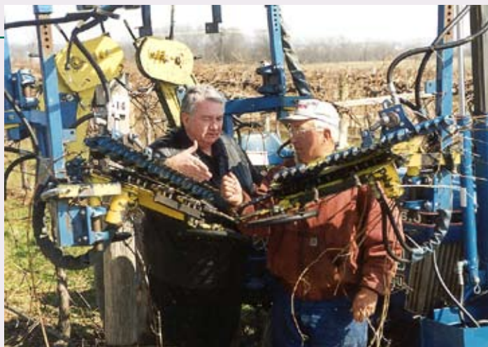
PRUNER — Justin Morris, left, and Tom Oldridge examine the prototype of a pruner that is part of the patented Morris-Oldridge Vineyard Mechanization System.
