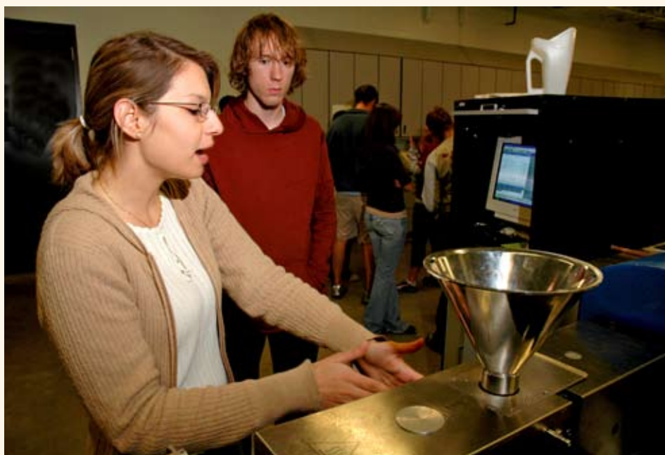
STUDENT RESEARCH DEMONSTRATION — Fernanda Onofre of Brazil explains the operation of an extruder to Will Gilbert of Mena, a fellow student in Fundamentals of Food Processing class. The extruder can process any kind of food into cereals and other products. Onofre uses the extruder in a student research project.
