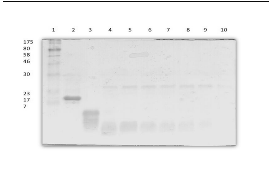
Figure 3. Chymotrypsin. Gel electrophoresis of chymotrypsin assay. Lane 1, molecular weight maker (kDa). Lane 2, Rheb. Lane 3, Chymotrypsin. Lane 4, 0 minutes. Lane 5, 1 minute. Lane 6, 5 minutes. Lane 7, 10 minutes. Lane 8, 20 minutes. Lane 9, 30 minutes. Lane 10, 60 minutes.
