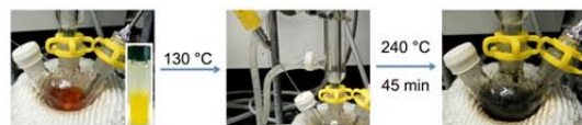
Figure 1. Reaction scheme for Pd,Fe nanocrystals. This was taken during the synthesis of Sample 1 prepared with Iron (II) Chloride tetrahydrate and Palladium (II) acetylacetonate. The left picture was taken at room temperature and the inset shows the W(CO) 6 solution. The middle was the injection and the right picture was taken at the end of the reaction at 240 °C.
