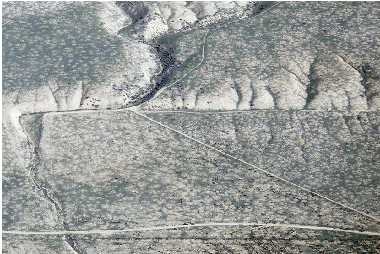
Figure 6.6: Aerial photograph of offset stream channels view northeast at Wallace Creek along the San Andreas Fault, Carrizo, California. Main channel is offset about 130 m and was incised around 3,700 years ago. Channel farther to the left on the near side of the fault was displaced about 250 m and was incised around 10,000 years ago. These offsets and ages indicate a long term slip rate of about 35 mm/yr along the San Andreas fault (Sieh & Jahns, 1984). Photo by (Rymer, 2013).
