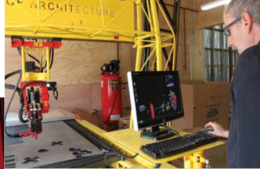
Santiago R. Perez operates the computer on this custom-made machine that does computer numerically controlled plasma cutting and five-axis milling.
