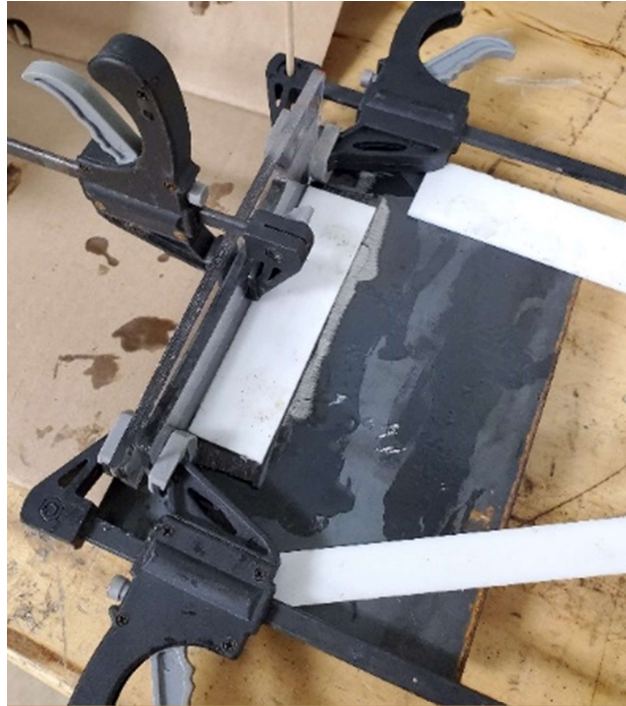
Figure 16. Layup method of CFRP showing clamps and acrylic molds
