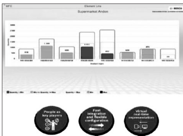
Fig. 10. Supermarket shows the maximum and minimum quantity of parts in real-time [13].
