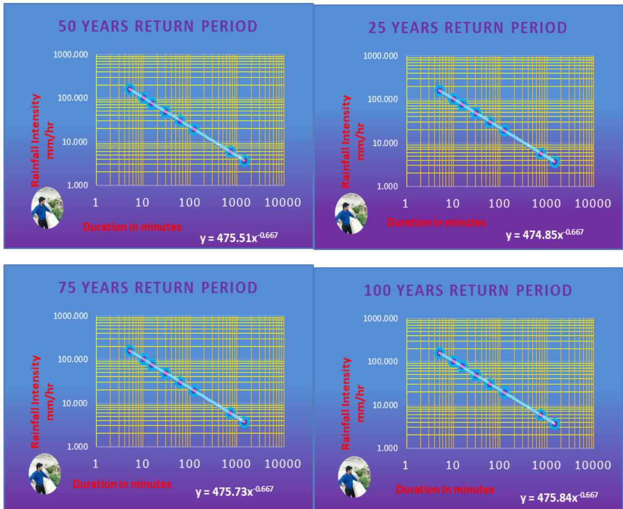
Figure 9 IDF curves for Hassan Station
