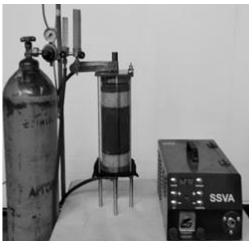
Figure 3. High-temperature unit for thermal treatment of carbon materials by TMEC
