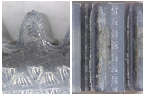
Fig. 17. PA66-CF gears with deformed teeth and wear on the flanks
