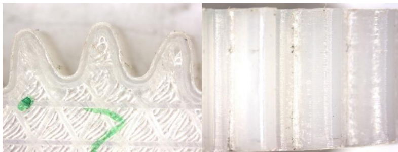
Fig. 16. PA66 gear after two Mio. cycles at a root stress \sigma_F = 12 \text{ MPa}
