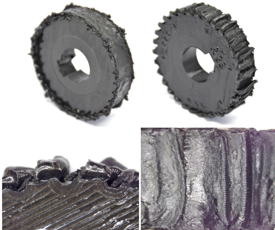
Fig. 14. PLA Gears with melted teeth
