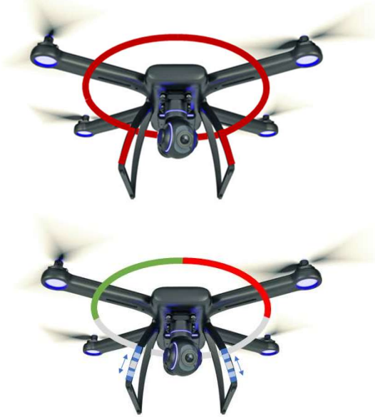
Figure 1: Top: Drone All-Round-Light Switched to Danger (Red). Bottom: All-Round-Lights Switched to Navigation
