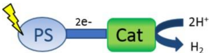
Figure 1. Schematic of a typical linked hydrogen evolution complex. In such a system, the PS represents a light-absorbing molecule called a photosensitizer and the Cat represents a hydrogen evolution catalyst.
