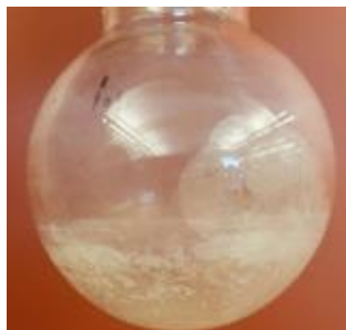
Figure 22. Oily white gum product formed from the purification of the reaction between 4,4'-dimethyl-2,2'-bipyridine with N -bromosuccinimide.
