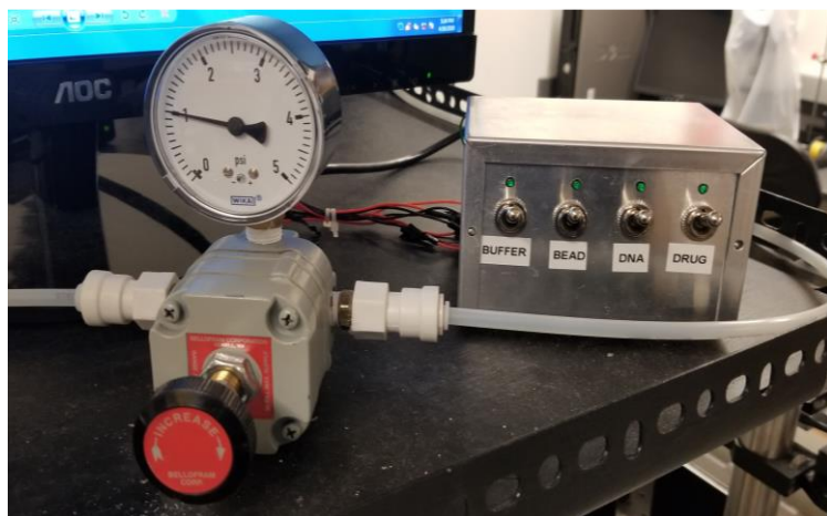
Figure 17: Electrical flow control box to control the flow of buffer, beads, DNA, and drug into the flow-cell. Compressed air is used to apply pressure on the biomaterials inside the reservoir to push them through the tubings into the flow-cell for the experiments.
