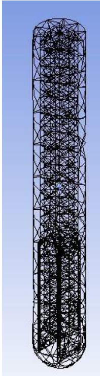
Figure 4.6 A mesh configuration for the viscosity probe surrounded by a fluid domain
