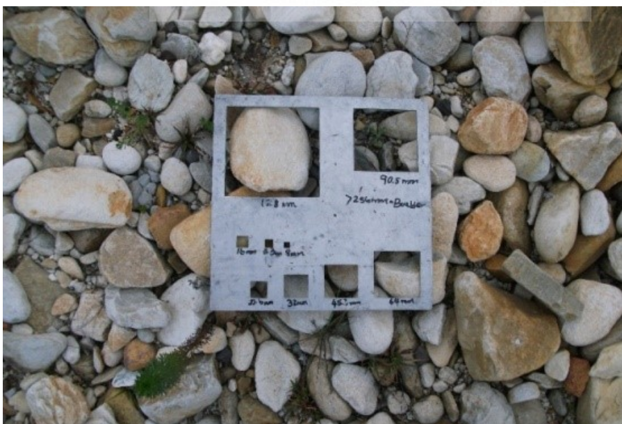
Figure 4.2: Image showing the gravelometer template used in the study.
