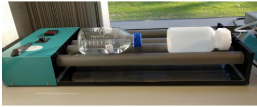
Figure 19 Polymer being mixed on a roller mixer
