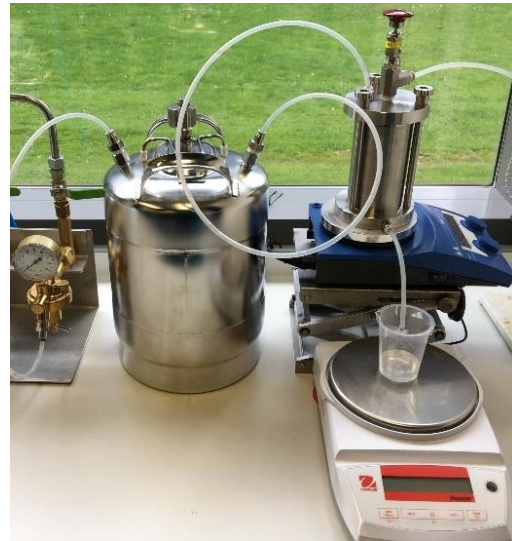
Figure 29 Image of the Amicon cell set-up including the dispensing vessel
