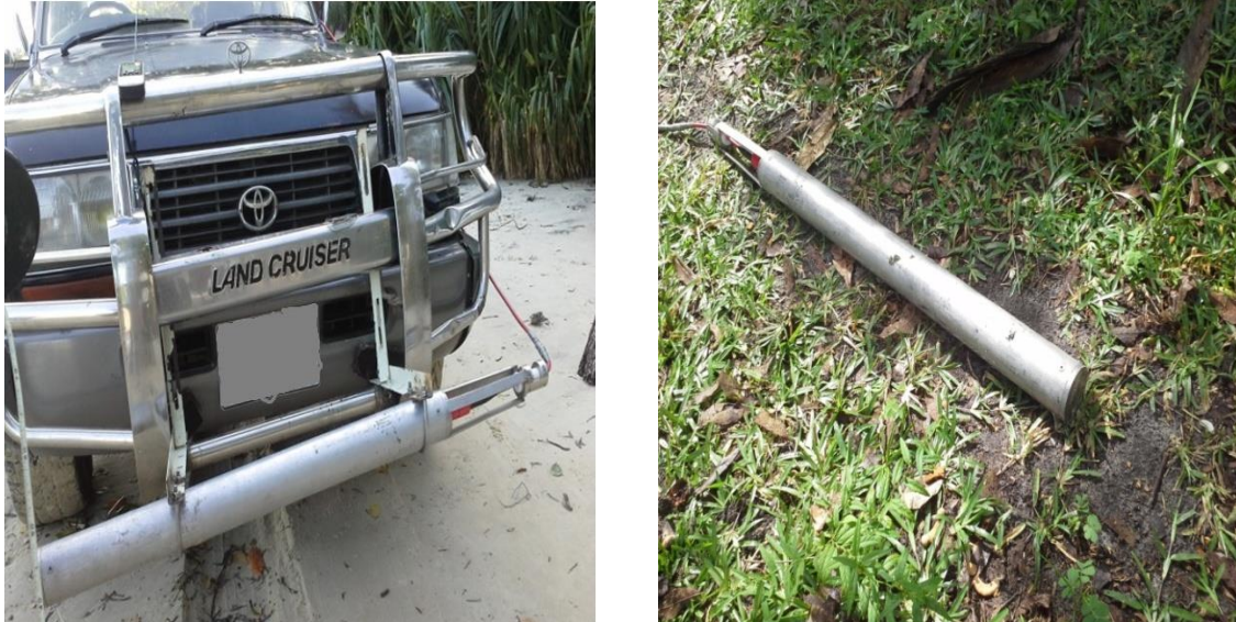
Figure 3.6: The ERL MEDUSA \gamma -ray detector system during in-situ gamma-ray mapping, mounted on a 4 x 4 vehicle at Kuku beach in Pemba (left) and placed on the ground at Msuka (right).
