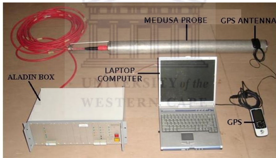
Figure 3.5: Components of the MEDUSA \gamma -ray detector system.
