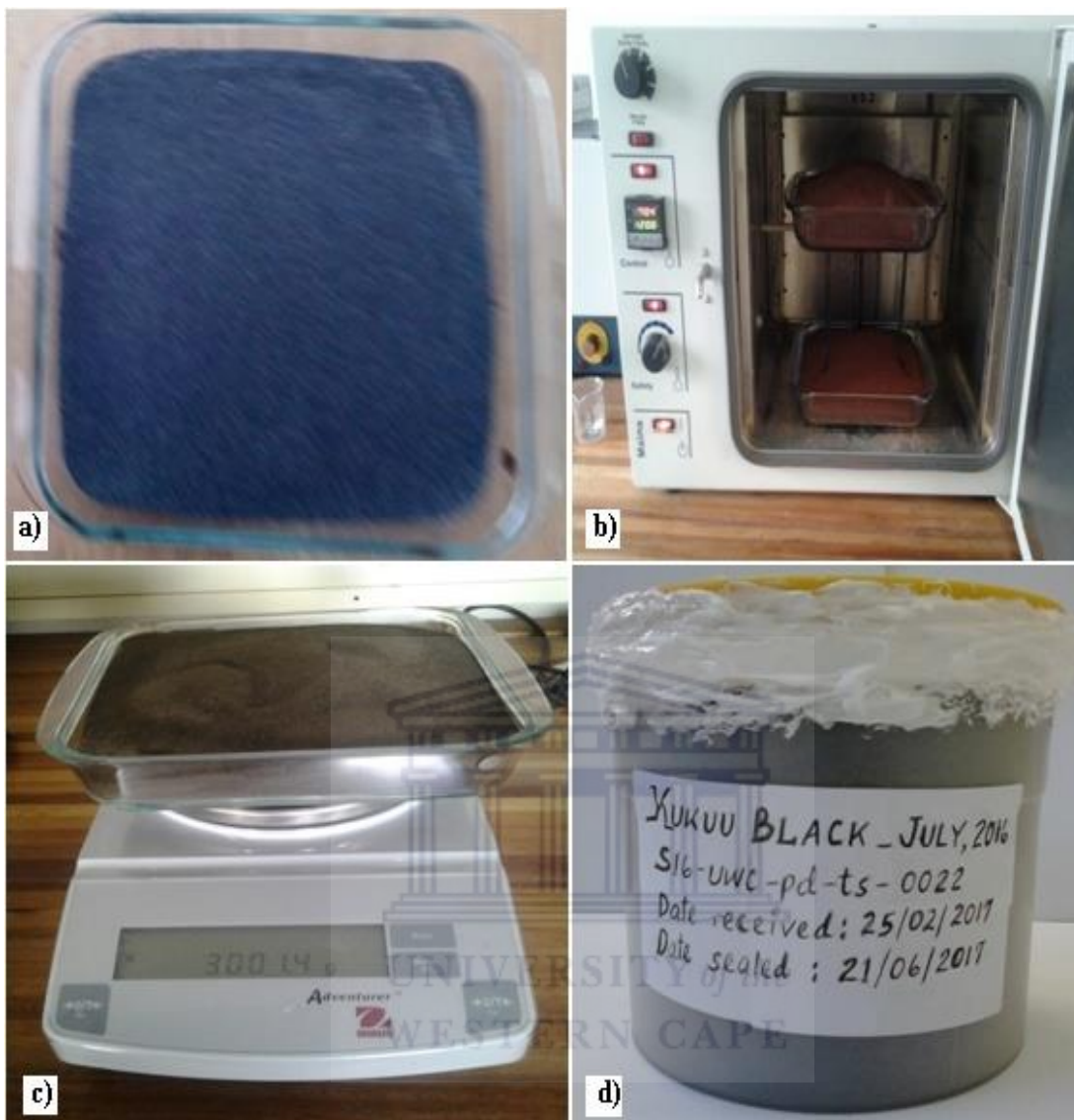
Figure 3.16: Soil and beach sand sediments preparations: a) Sample drying at room temperature b) Oven drying at 110°C c) Weighing a dried sample d) A prepared soil sample in the Marinelli beaker.
