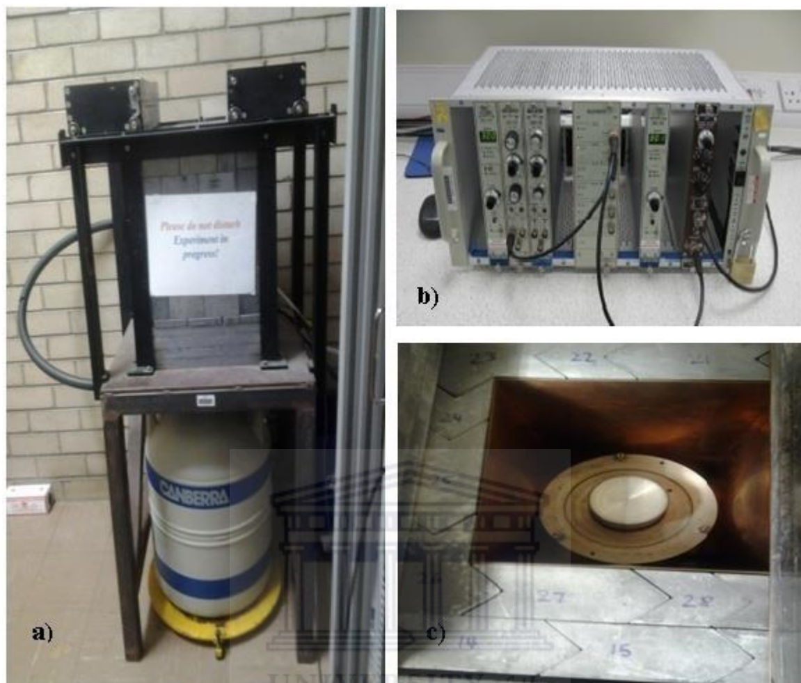
Figure 3.17: A picture showing components of the HPGe detector system used in this study: a) The lead castle and the liquid nitrogen Dewar, b) the NIM power supply c) the top of the detector
