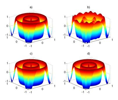
Figure 2.8 The spectral filtering of  $u = \cos(4\pi\sqrt{x^2 + y^2})$  in Q space by eliminating higher frequency orthogonal hull basis Eq. (2.34). a)  $k_m = 400$ , i. e. full rank, b)  $k_m = 200$ , i. e. half rank, c)  $k_m = 360$ , i. e. ninety percent rank, d) Exact
