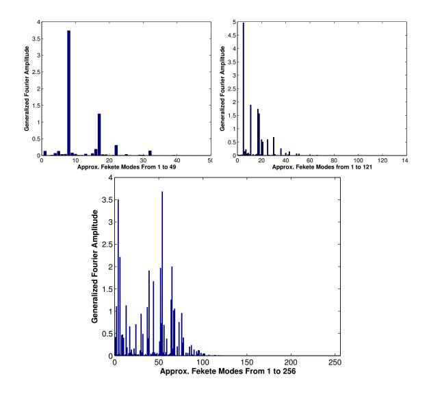
Figure 2.13 The spectra of  $u = \sin(\pi x) \sin(\pi y)$  on different convex/concave elements; Left) using 7<sup>th</sup> order orthogonal spectral hull basis  $\bar{\Psi}$  on a quadrilateral element. Right) using 11<sup>th</sup>  $\bar{\Psi}$  on a hexagonal element. Bottom) using 16<sup>th</sup>  $\bar{\Psi}$  on a T-shape element
