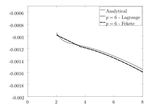
Figure 4.19 v solution comparing p=6 Lagrange and p=6 Fekete techniques with analytical solution
