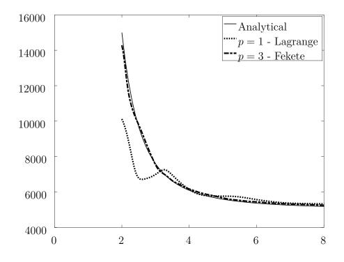
Figure 4.22  $\sigma_x$  solution comparing p = 1 Lagrange and p = 3 Fekete techniques with analytical solution where x = 0
