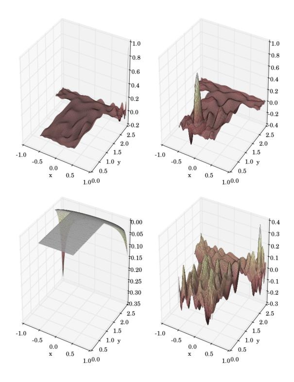
Figure 2.9 The first and the 200th shape functions of *nodal* (top) and *modal* (bottom) Approx. Fekete basis. Top Left)  $\psi_1$ , Top Right)  $\psi_{200}$ , Bott. Left)  $\bar{\psi}_1$ , Bott. Right)  $\bar{\psi}_{200}$
