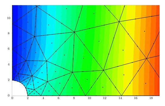
Figure 4.3 u solution on p = 3 grid with Lagrange Basis
