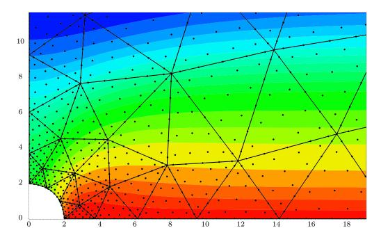
Figure 4.10 v solution on p = 6 grid with Fekete Basis
