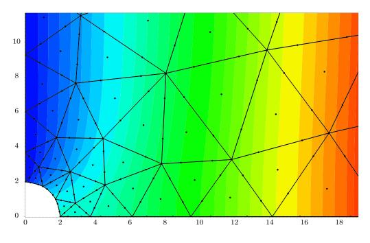
Figure 4.7 u solution on  $p=3~{\rm grid}$  with Fekete Basis
