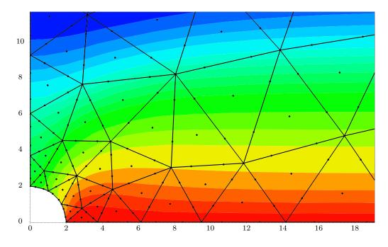
Figure 4.8 v solution on p = 3 grid with Fekete Basis
