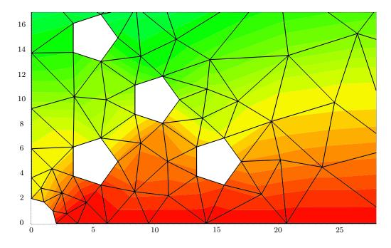
Figure 4.29 v solution of Complex Geometry data using p = 1 Lagrange technique
