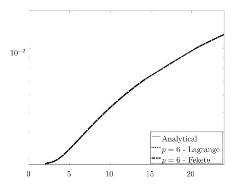
Figure 4.18 u solution comparing p = 6 Lagrange and p = 6 Fekete techniques with analytical solution (semi-log y plot)
