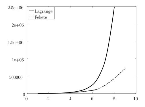
Figure 4.21 Comparison of Matrix condition number of higher order FEM methods utilizing Lagrange and Fekete techniques
