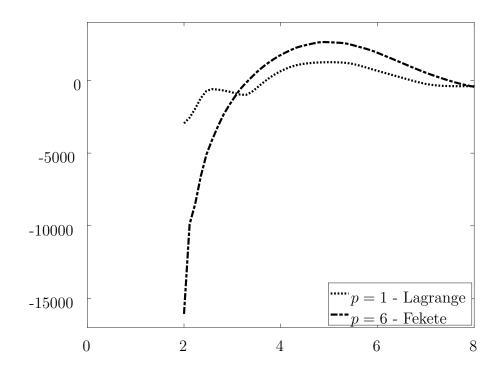
Figure 4.31  $\sigma_y$  solution of Complex Geometry data comparing p=1 Lagrange and p=6 Fekete techniques where y=0
