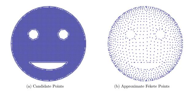
Figure 2.3 The procedure of generating candidate points (a) and selecting approximate Fekete points (b) on a concave hull
