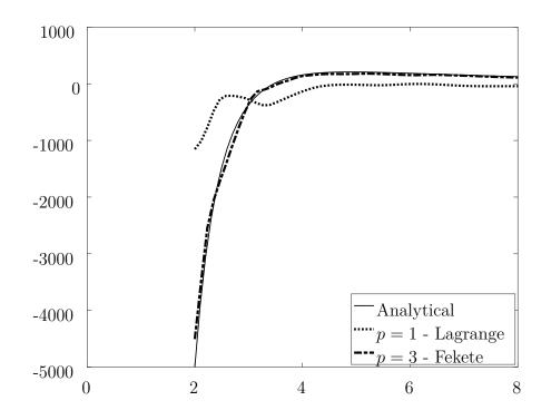
Figure 4.23  $\sigma_y$  solution comparing p = 1 Lagrange and p = 3 Fekete techniques with analytical solution where y = 0
