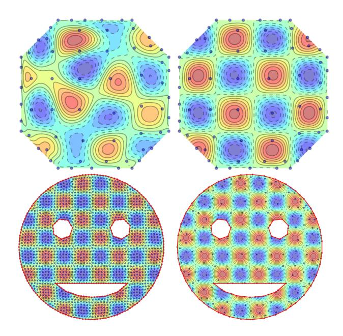
Figure 2.10 Comparison of spectral hull basis functions and RBF in the reconstruction the solution on a hull. Top row) with same DOF, Bottom row) with same  $L_2$  error, Left column is RBF, right col. corresponds to orthogonal spectral hull basis functions  $\bar{\Psi}$
