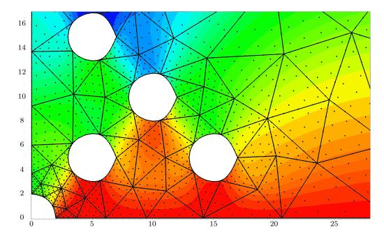
Figure 4.27 v solution of Complex Geometry data using p = 6 Fekete technique
