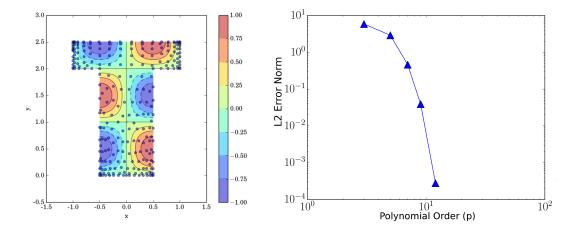
Figure 2.12 Superlinear convergence of spectral hull basis on the concave T-hull. Left) Reconstructed function using  $16^{th}$ -order spectral hull basis constructed on approximate Fekete points. Right)  $L_2$  error compared to analytical reconstruction
