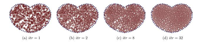
Figure 2.2 The generation of the candidate points using a pseudo time iterative gravitational method
