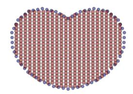
Figure 2.1 The generation of the candidate points using the fill pattern method
