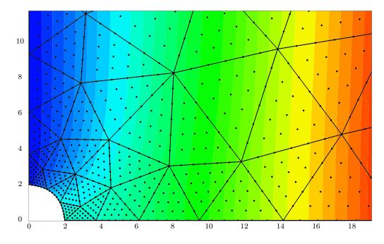
Figure 4.5 u solution on p = 6 grid with Lagrange Basis
