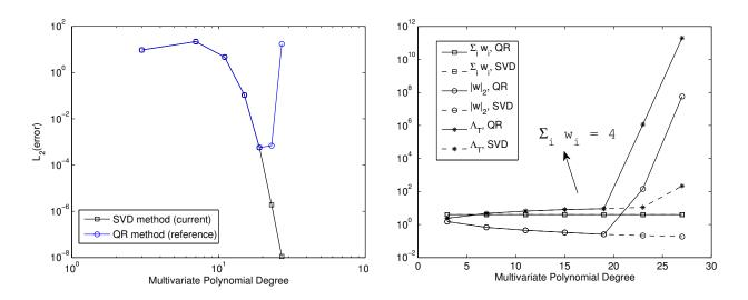
Figure 2.4 The comparison between SVD and QR approaches to find approximate Fekete points using only one iteration. Left) The interpolation error versus polynomial degree, Right) Various measures
