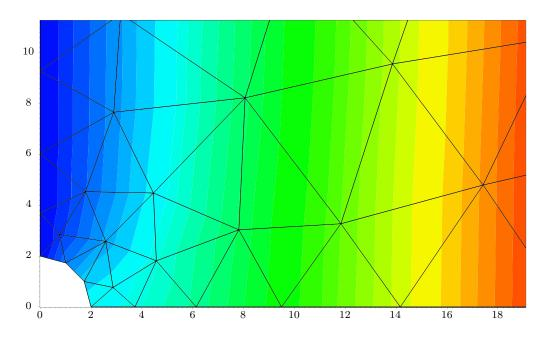
Figure 4.1 u solution on p = 1 grid with Lagrange Basis
