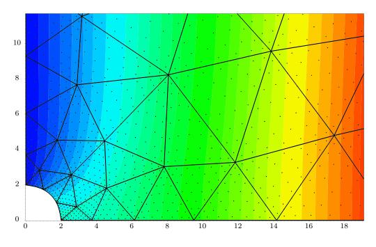
Figure 4.11  $\boldsymbol{u}$  solution on p=9 grid with Fekete Basis
