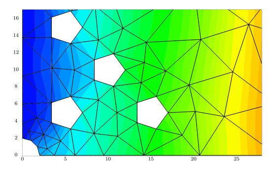
Figure 4.28 u solution of Complex Geometry data using p = 1 Lagrange technique
