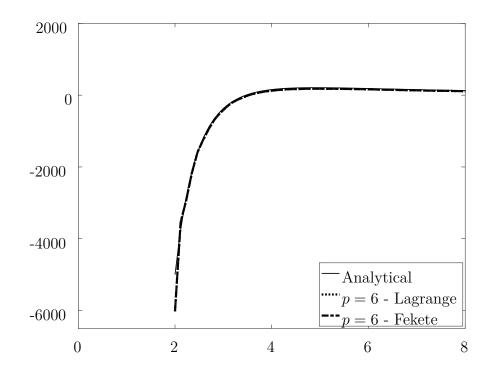
Figure 4.25  $\sigma_y$  solution comparing p = 6 Lagrange and p = 6 Fekete techniques with analytical solution where y = 0
