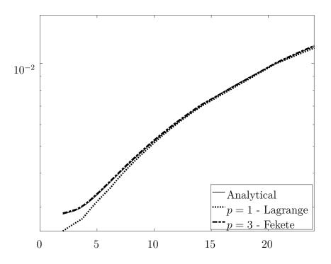
Figure 4.14 u solution comparing p=1 Lagrange and p=3 Fekete techniques with analytical solution (semi-log y plot)
