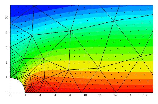
Figure 4.6 v solution on p = 6 grid with Lagrange Basis
