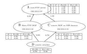
Example of BAG – attacker (D) can use two buffer overflow exploits (B, C) to get access to a server (A)
