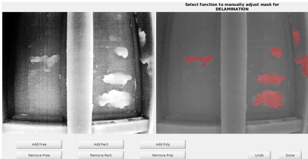
Figure C.4: Figure showing the final mask (red shows defect pixel labels) overlaid over the original image after manual intervention. Manual intervention was able to remove objects that appeared bright but were not a delamination and was also able to fill in any remaining gaps in the delamination areas.
