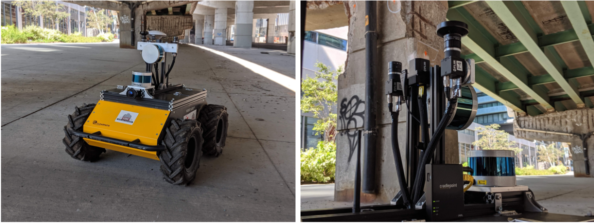
Figure 4.2: Husky Inspection platform. (Photos by: Nicholas Charron)
