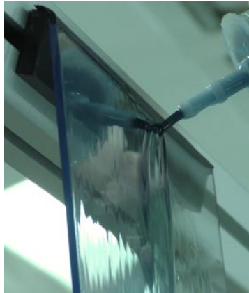
Picture 21. Common flow coating process. [47]
