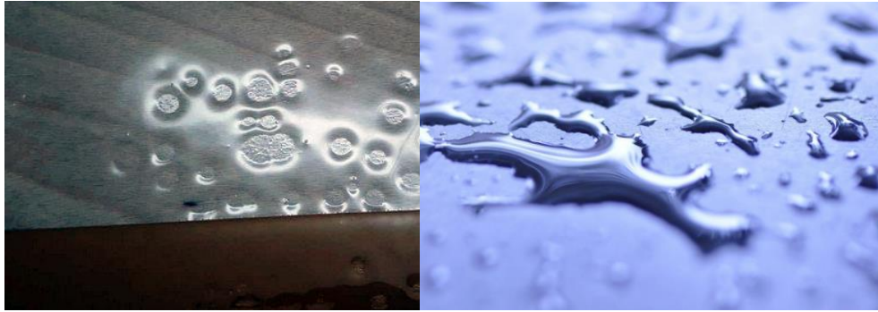
Picture 4. The fisheyes effect on left and crawling/dewetting effect on the right. [16]
