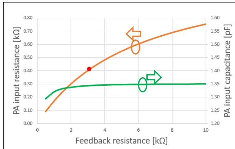
Figure 38: PA input impedance modified by the resistive feedback.
