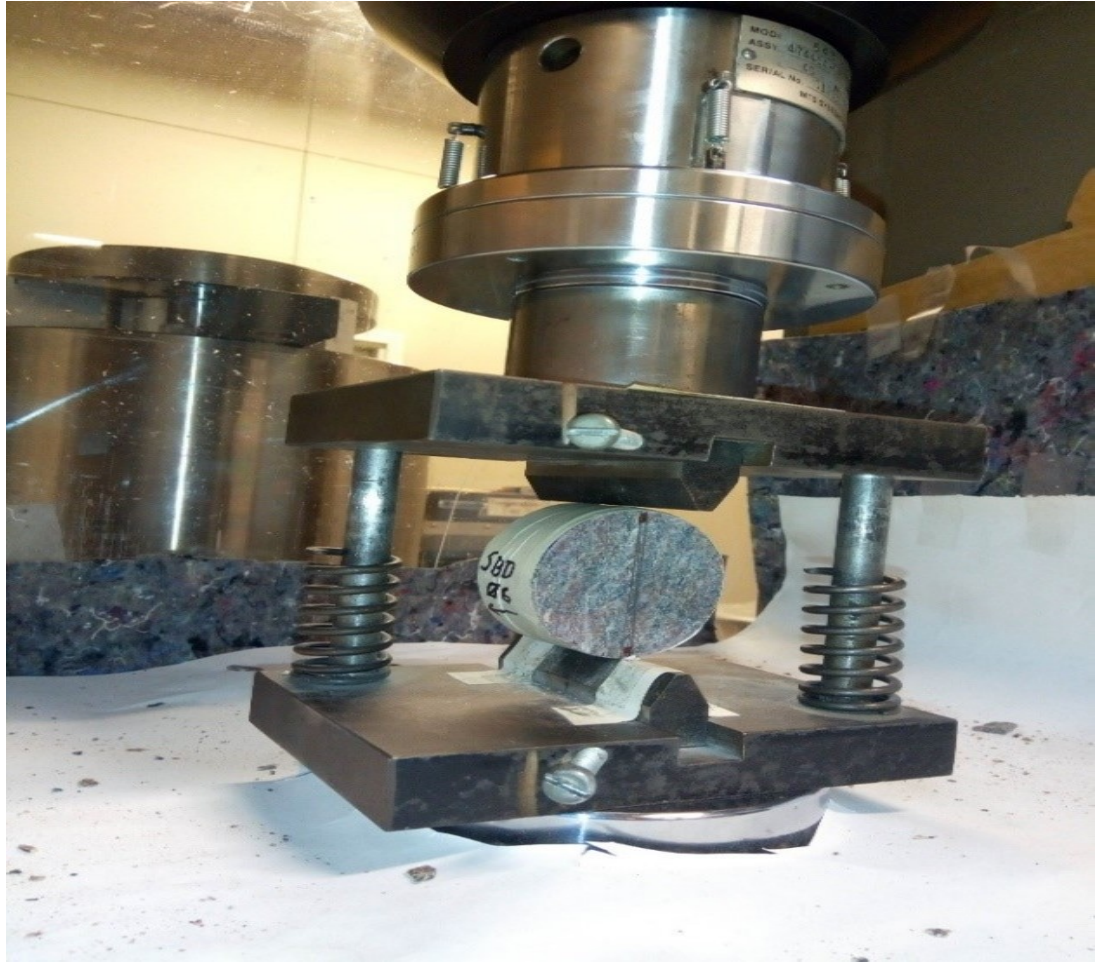
Figure 3.8. A specimen wrapped with a masking tape for BTS test.
