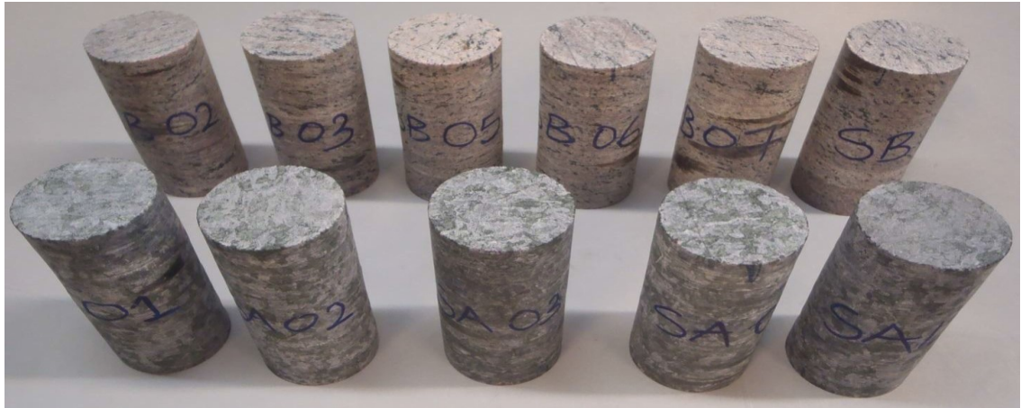
Figure 3.4. Cylindrical uniaxial compression test specimens after re-grinding (photographed by P. Eloranta, Aalto ENG)
