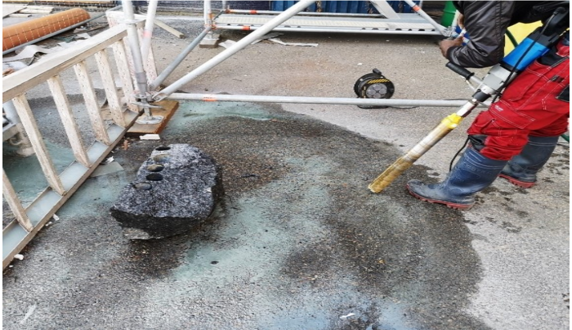
Figure 3.2. Drilling core samples from the boulders drilling at the Oulu Mining School (OMS) (photographs by Kimmo Kärenlampi)
