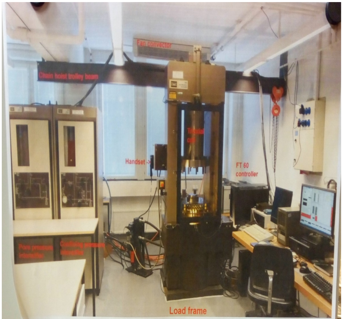
Figure 3.6. MTS 815 Rock mechanics test system
