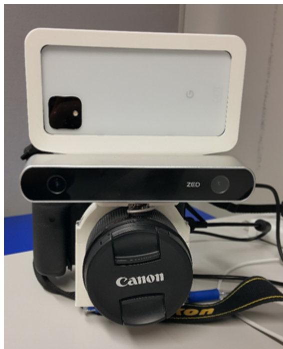
Figure 19. The multi-Camera rig. The components of the rig are as the following: Pixel4 mobile camera on the top, ZED stereo camera in the middle, and Canon DSLR camera in the bottom.
