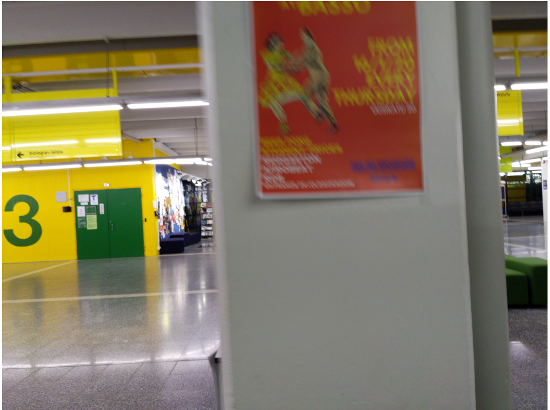
Figure 5. Image with depth-dependent blur. The foreground poster is significantly blurred, while the background is almost sharp.
