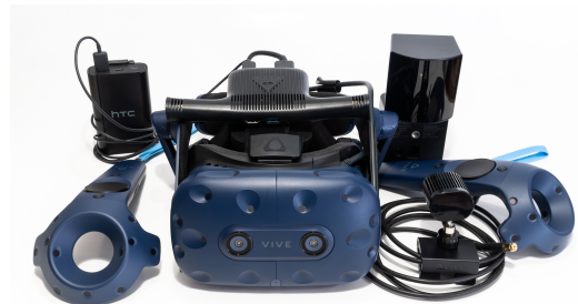
(e) Components of HTC Vive Pro VR system with wireless adapter. PCI-E expansion card of the wireless transmitter is not shown in the image. Also, power cords for the base stations are excluded from the image for clarity.
