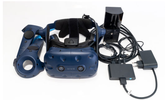
(d) Components of HTC Vive Pro VR system. Power cords for the base stations are excluded from the image for clarity.
