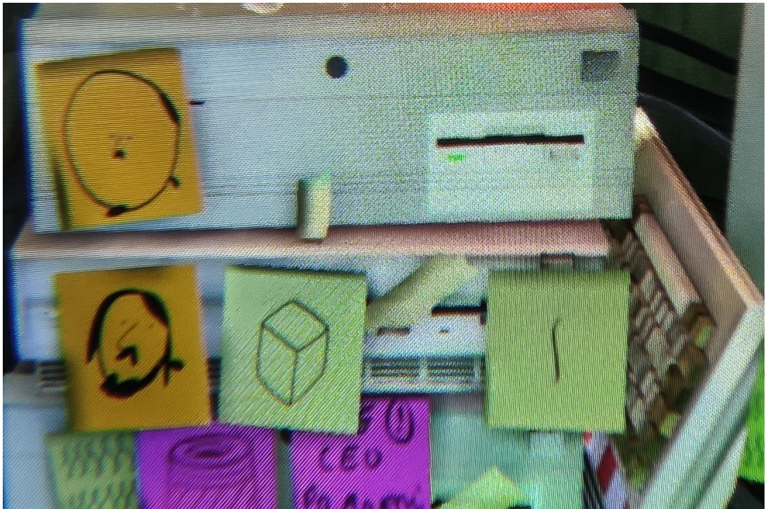
Figure 2. Effects of low resolution and screen door effect in an HMD's image.
