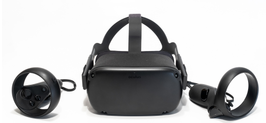
(a) Components of Oculus Quest VR system. Charger is excluded from the image.
