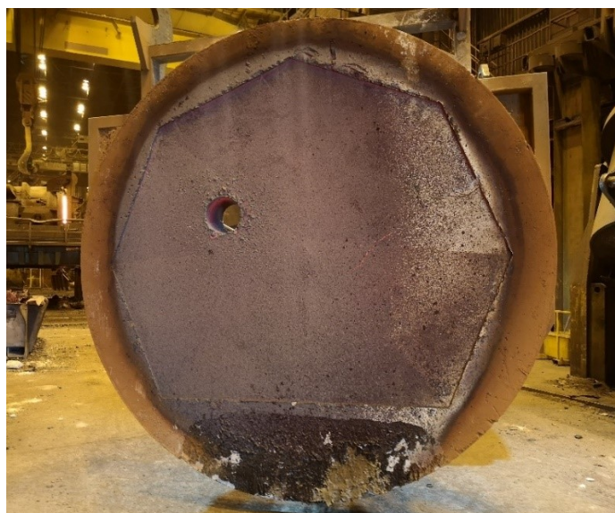
Figure 53. Experimental lining made with single cast.
