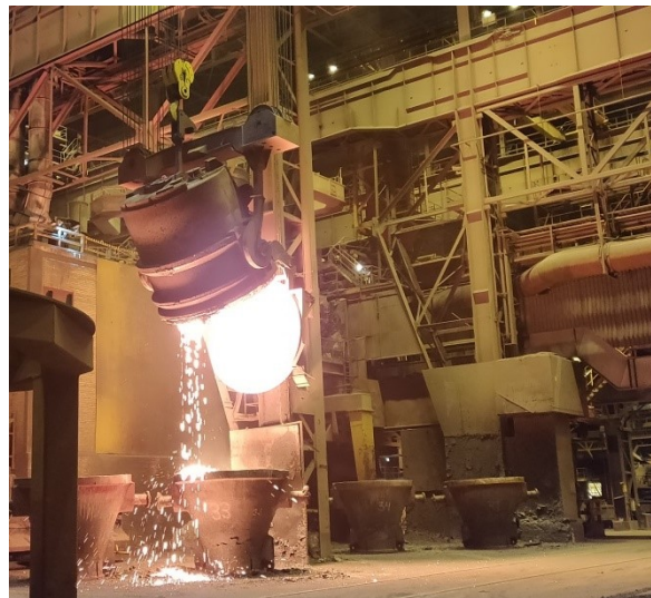
Figure 7. Lid remains attached to the ladle during slag pouring.
