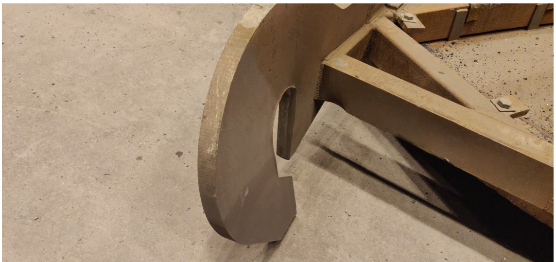
Figure 38. Hinges are usually bent if a lid falls off a rack.
