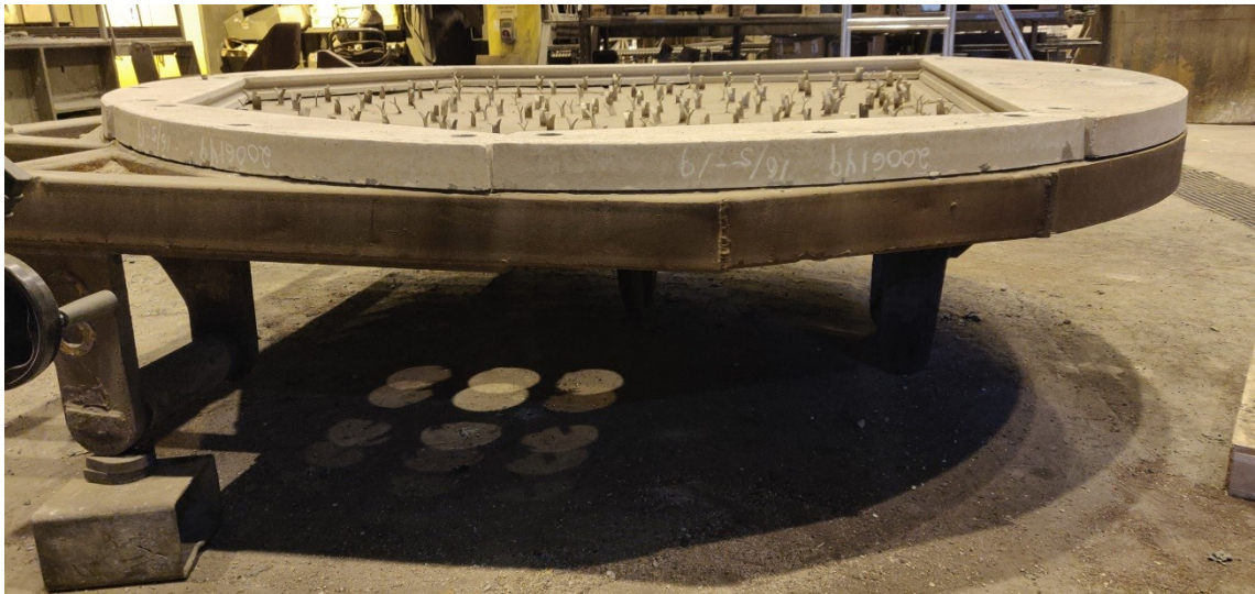
Figure 39. Lid has been crooked as a result of continuous maltreatment.
