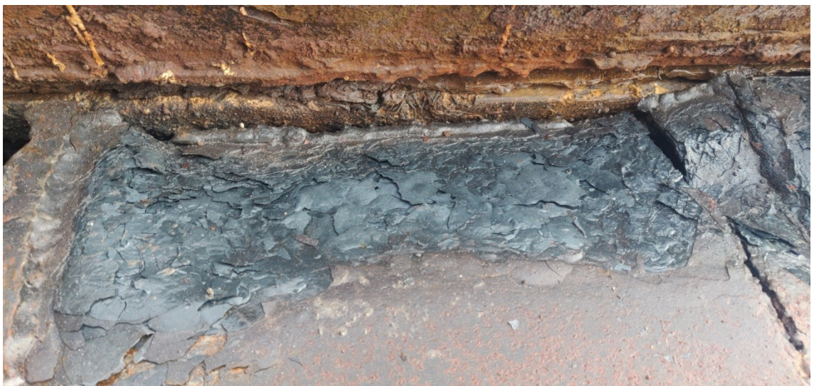
Figure 34. Repeating exposure to the heat makes metal structure to lose its shape and strength.
