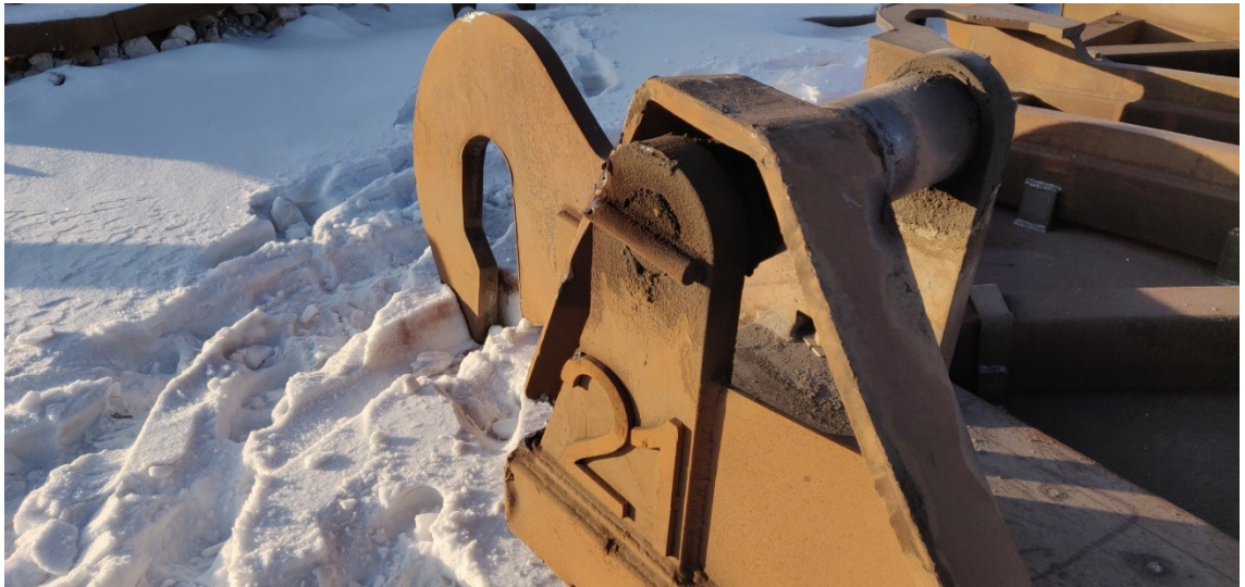
Figure 37. Protective guardrail of the bearing has bent as a result of impact.
