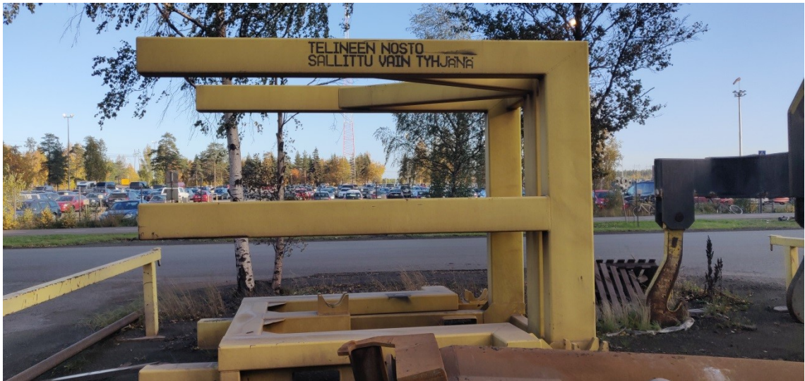
Figure 12. Storing rack for steel ladle lids.
