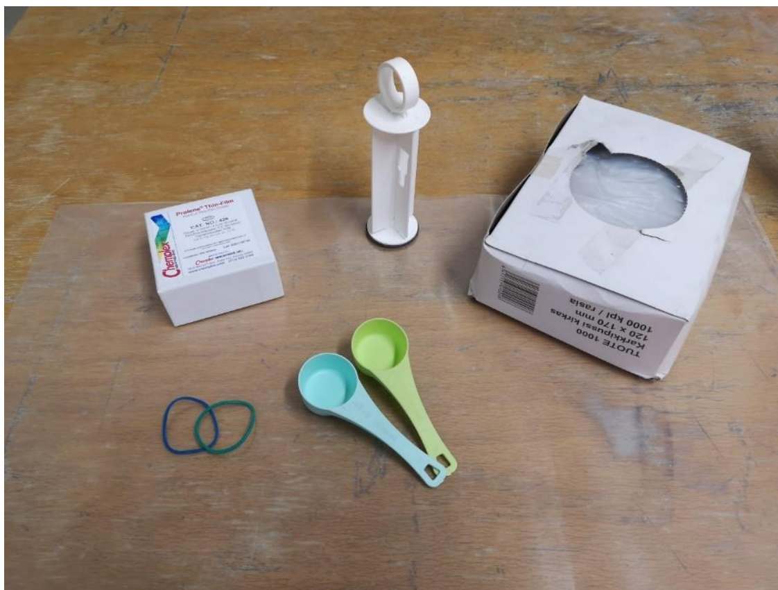
Figure 5. Sample preparation tools: 15 ml measuring spoons, rubber bands, candy bags, a syringe presser and Prolene ® thin films.
