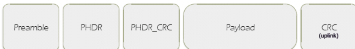
Figure 12. Message structure of LoRaWAN physical layer.
