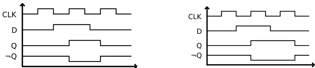
Figure 2.11. Timing diagram of D-latch (left) and D-flip-flop (right). CLK is clock of the circuit, D is an input, Q is an output and \neg Q is inverse of Q.
