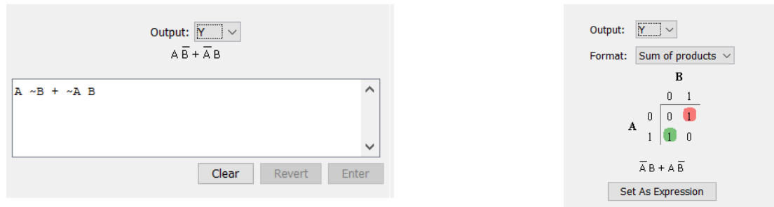
Figure 3.4. Logisim expression (left) and Karnaugh map (right) of Figure 3.2. circuit.
