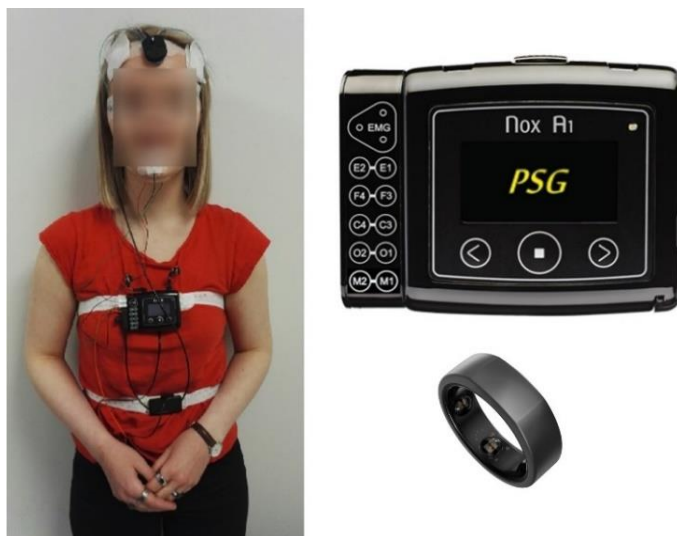
Figure 4. Electrode layout, Nox A1 and Oura ring.
