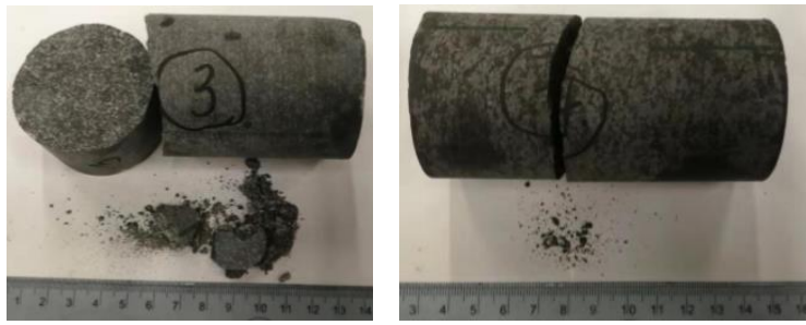
Figure 13. Rock samples a) Sufficiently broken OMS-19-2 and OMS-19-11, b) not-sufficiently broken OMS-19-6 and OMS-19-15, c) broken at the weakness zone OMS-19-3 and OMS-19-7.
