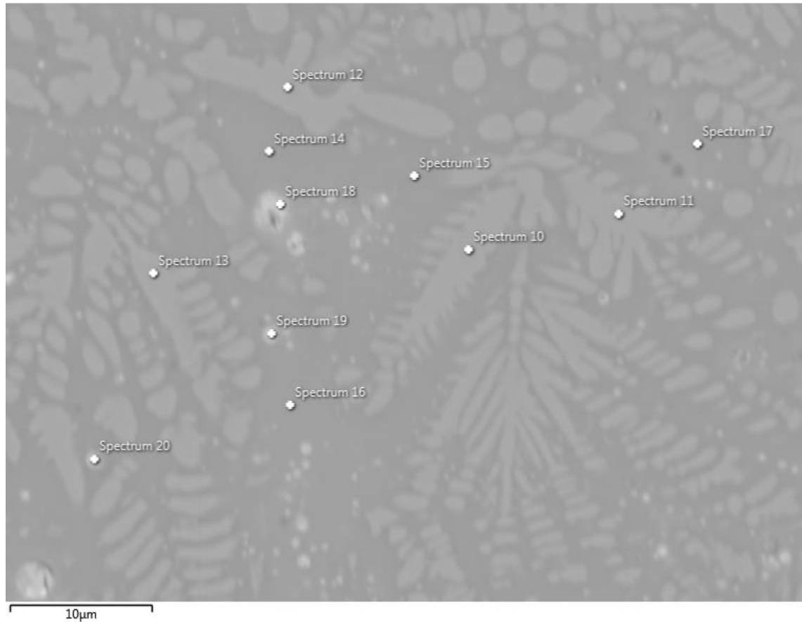
Figure 14. FESEM image of dendritic structure near the edge of the sample.
