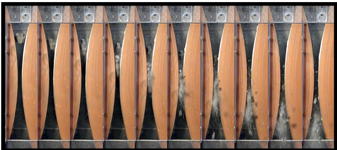
Picture 34. A particle breakage event in a series of high-speed photographs.
