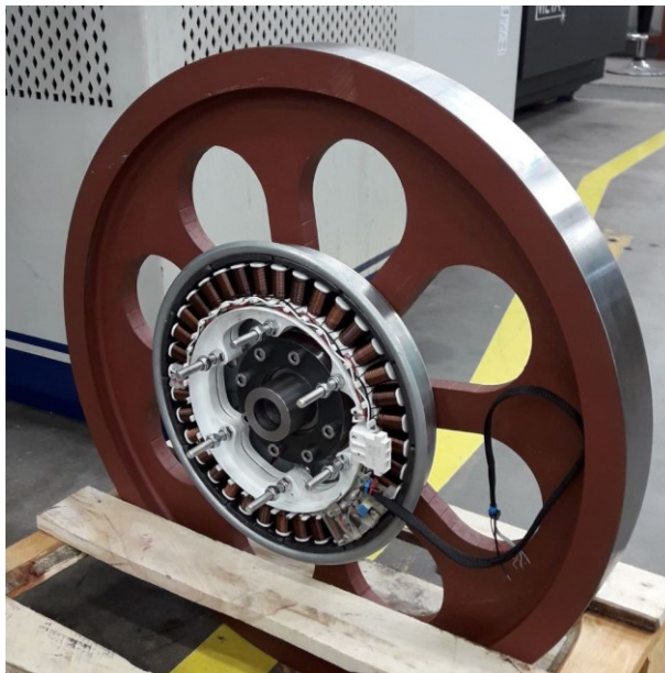
Picture 18. A washing machine motor installed on the finished crusher wheel.
