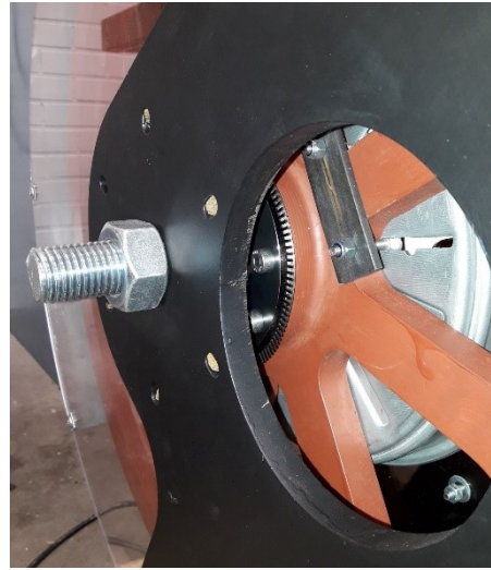
Picture 24. Optical encoder ring installed on the wheel hub.
