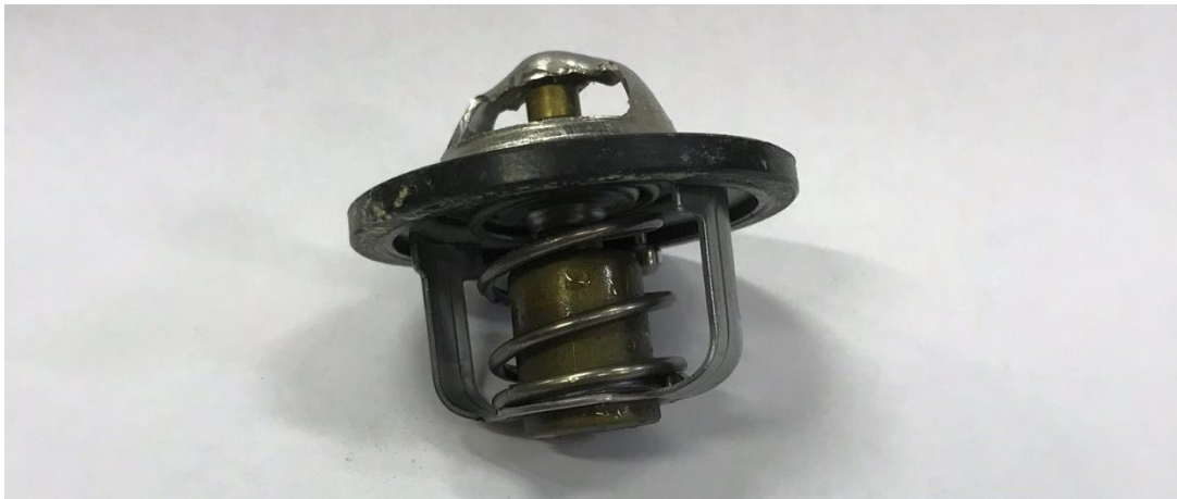
Figure 7. Thermostat construction by Yamaha from MT-07.
