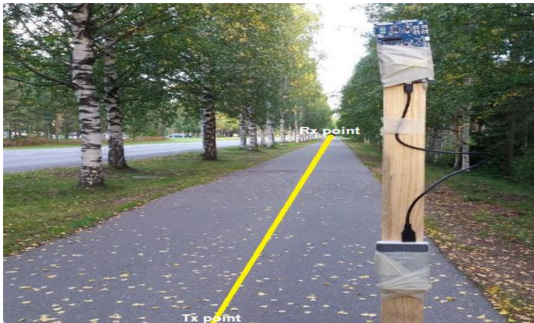
Figure 22. Outdoors LOS measurements (straight bicycle road).
