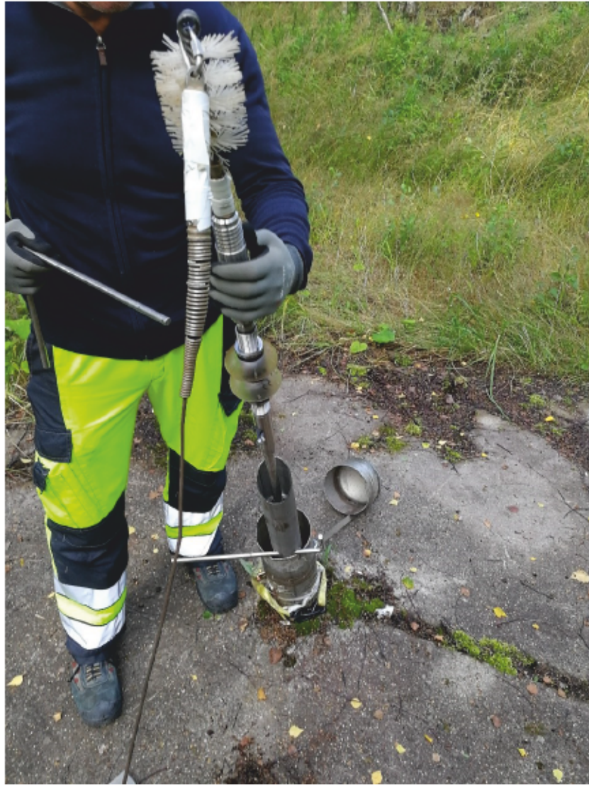
Figure 15. PFL Dummy installations on OL-KR42 in August 2019. In the upper part is the brush which is supposed to remove the drillhole debris etc. from the drillhole. Fallen off debris is collected to small container and is documented separately in each Dummy run.
