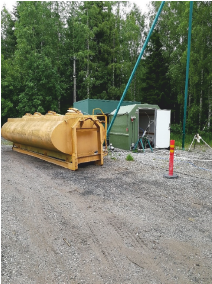
Figure 19. The overpressure system at OL-KR6 during 13–20 June. The orange tank is full of marked water that was pumped into OL-KR6.
