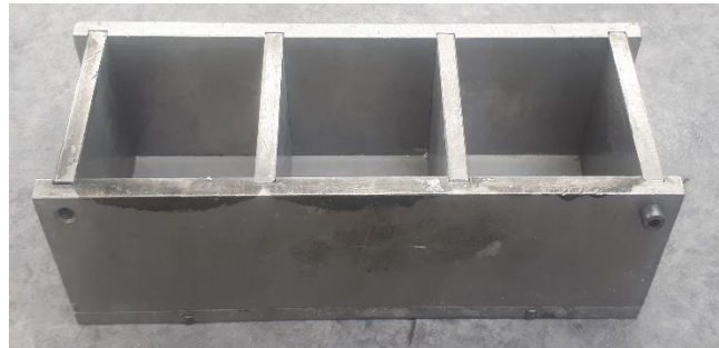
Fig 4 .5×5×5 molds used to make the samples.
