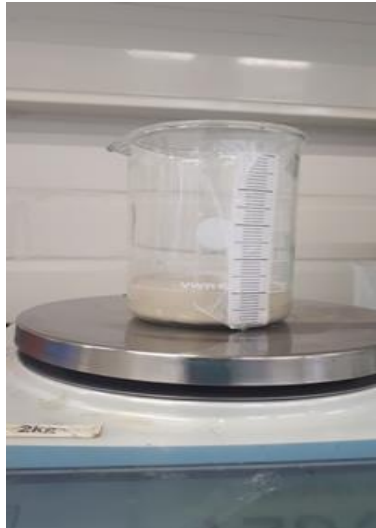
Fig 5. Arrangements to measure the fresh properties (Fresh density and Aeration rate).
