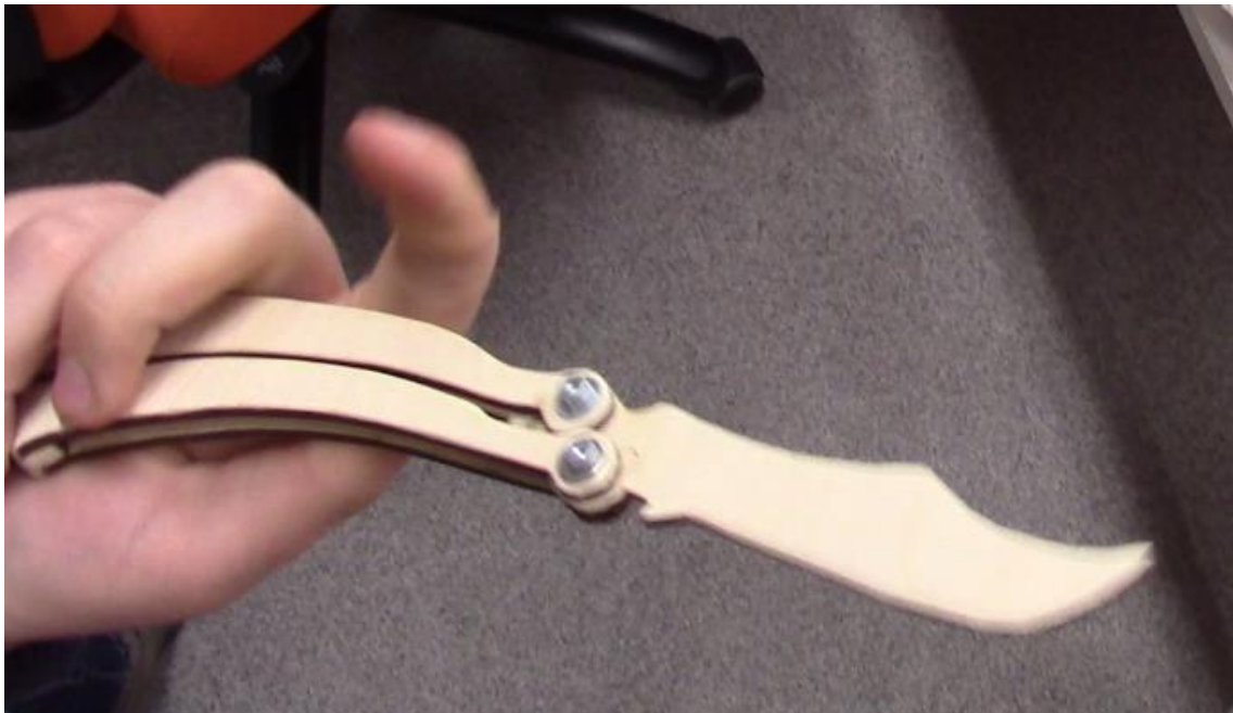
Picture 13. Butterfly knife from a videogame made by laser cutting by an attendee.
