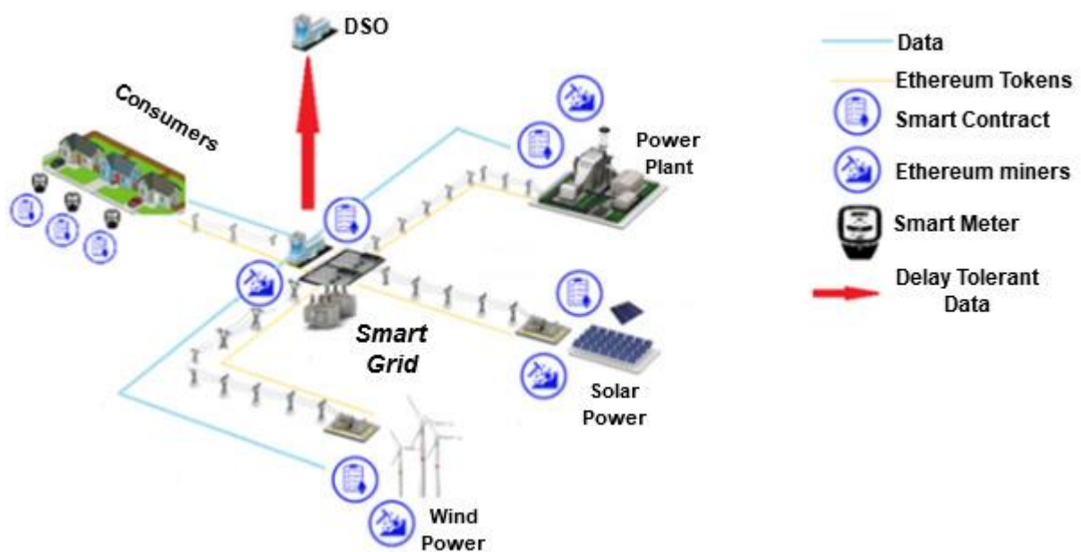
Figure 5. Blockchain-based smart grid using Ethereum
