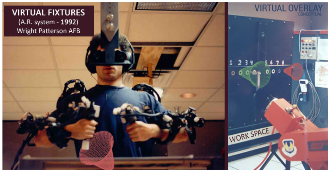
Figure 16. Virtual fixtures used to increase user performance in the task of telerobotic control of Fitt’s Law peg-board 2 .
