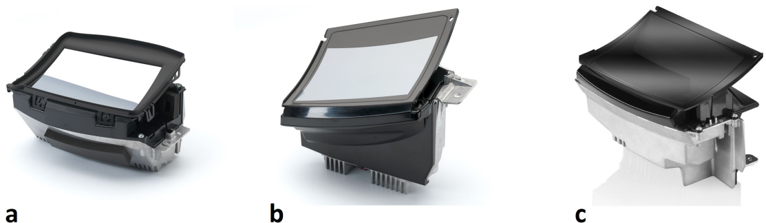
Figure 11. Continental Head-up Displays for Audi, BMW and Mercedes-Benz
