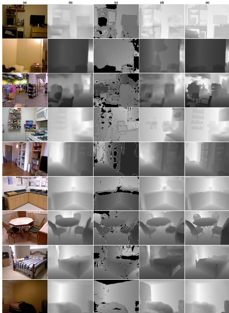
Figure 33. Depth map prediction of the supervised (column b) and unsupervised (column c) DepthNets on the NYU Depth v2 compare with Liu et al. [10] (column d). Column (a) and (e) show the input RGB and ground truth depth images, respectively.
