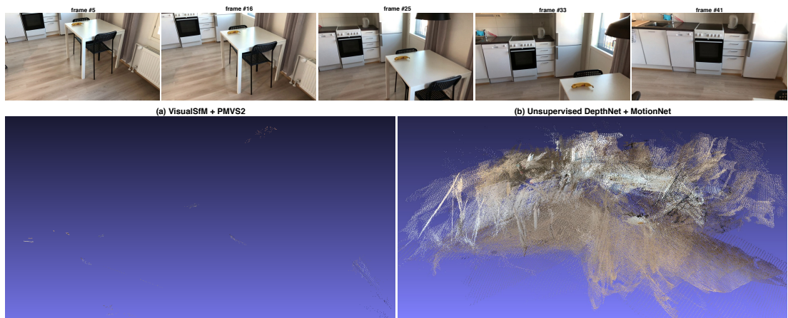
Figure 36. Reconstructed 3D point clouds from a real world dataset. The top row shows five input frames of the 60 total frames. Point cloud (a) was created using VisualSfM [2], which failed to reconstruct the scene. The learning based approach instead, was able to get a rough structure of the scene as shown in point cloud (b).
