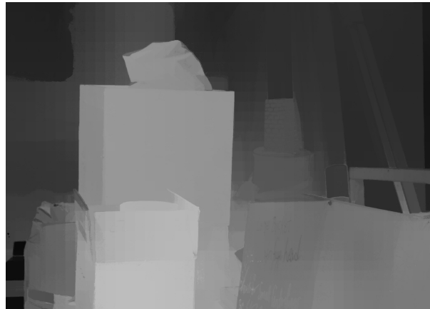
Figure 24. The depth map of the image Storage after the Fast Bilateral Solver.
