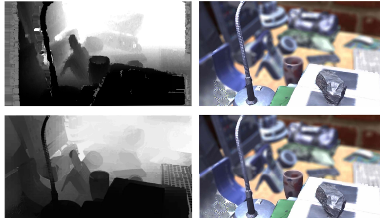
Figure 2. A comparison showing the difference between an unfiltered disparity map and its final result (above), and one filtered with Fast Bilateral Solver and its final result (below).
