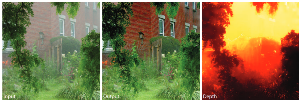
Figure 13. Dehazing based on a single input image and the corresponding depth estimate.
