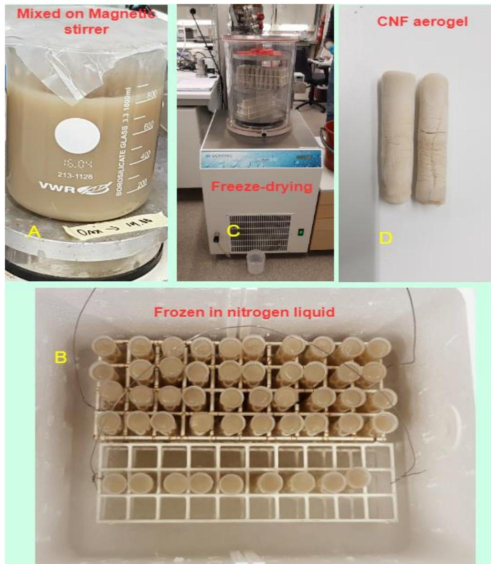
Figure 8. A) Illustration of CNF suspension stirred on a magnetic stirrer. B) CNF suspension frozen in a liquid nitrogen. C) Freeze-drying to obtain hydrophobized CNF aerogels. D) Prepared CNF aerogels.
