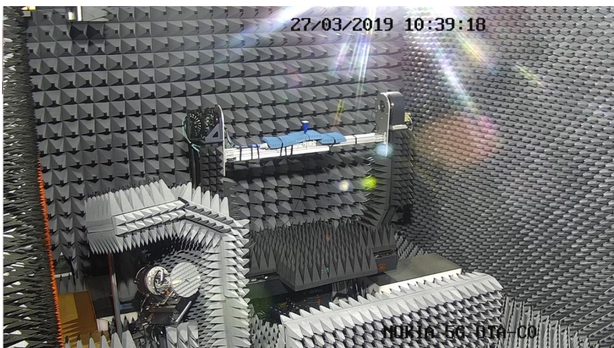
Figure 27. Calibration installation setup of SGH 2650-40.
