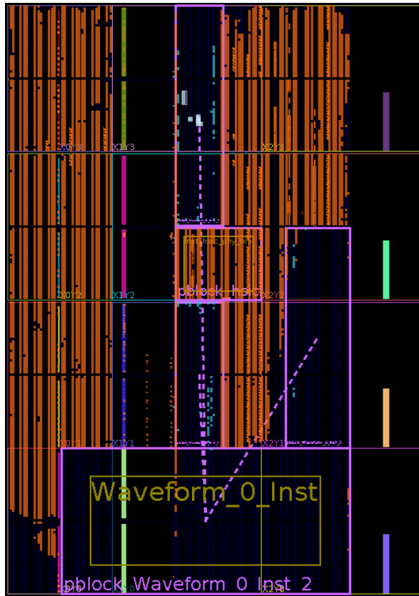
Figure 11. FPGA layout with greybox RM.
