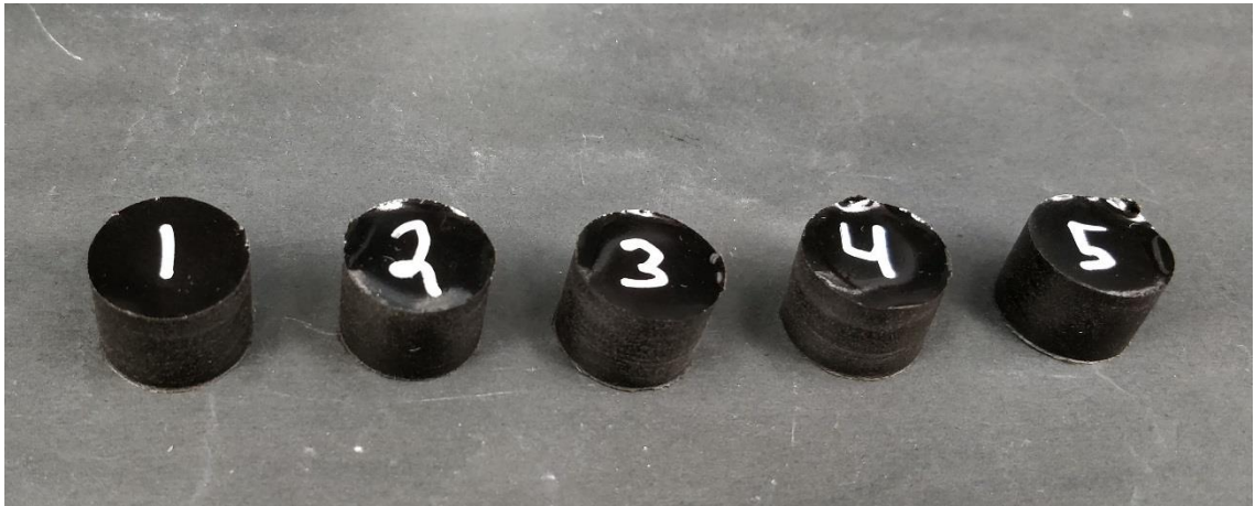
Figure 14. Abrasion test specimens before testing.
