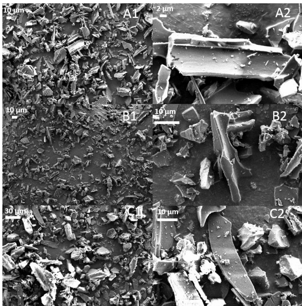
Figure 11. SEM images of pin-milled biochar samples. A1 and A2 are images of aspen samples, B1 and B2 birch samples, and C1 and C2 pine samples.
