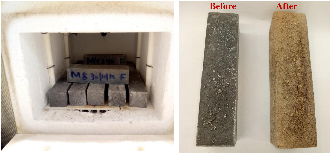
Fig 15. High-temperature exposure: (a) Specimens inside the oven; (b) After exposure to high temperature.
