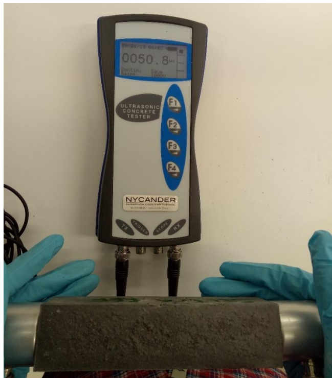
Fig 14. Measuring ultrasonic pulse velocity.
