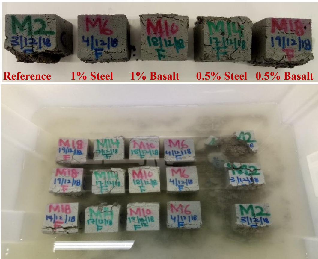
Fig 29. Reinforced mixtures with 5% lime during water absorption test.
