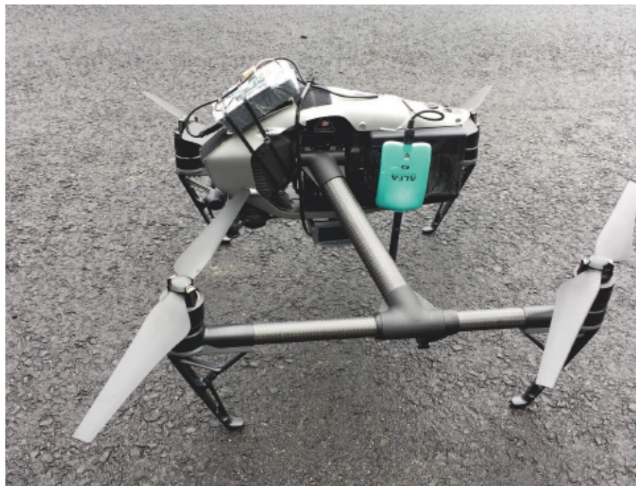
Figure 7. The Pi setup attached on drone.
