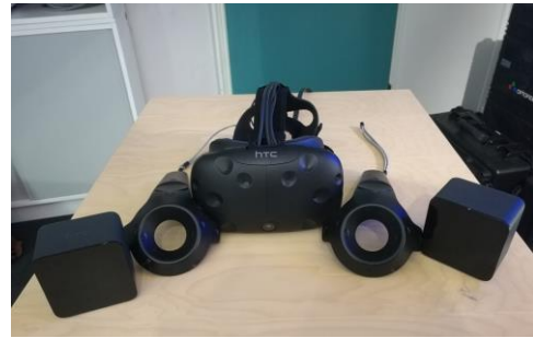
Figure 2. HTC Vive HMD, HTC Vive base stations and HTC Vive controllers. Picture taken by thesis group.
