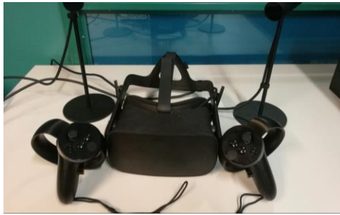
Figure 1. Oculus Rift HMD, Oculus sensors and Oculus Touch controllers. Picture taken by thesis group.
